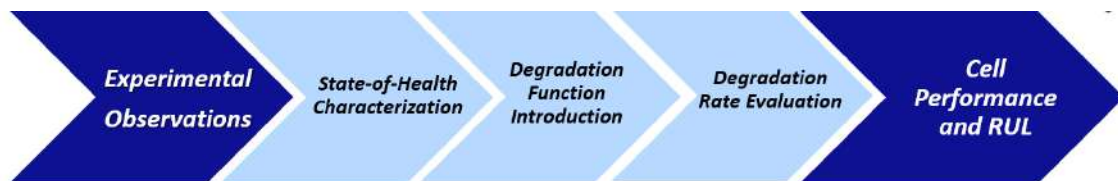
Figure II.1 UNIGE activity performed steps from nominal cell characterization to RUL estimation through SIMFC/SIMEC.
